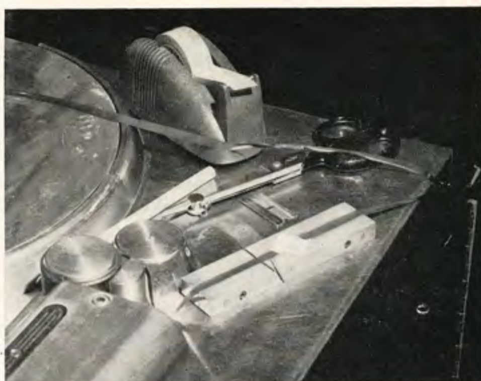
Fig. 5. Tape ends are joined together in the splicing block. The #41 Scotch tape is applied at an angle to the magnetic tape so there will be the least possible disturbance to smooth motion of the tape through the head assembly.
