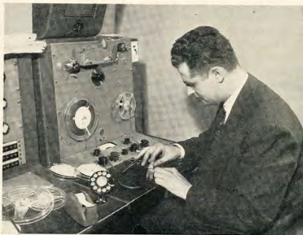
Fig. 8. Tape editor A. J. Sisco splicing tape at NBC cutting room. (NBC photo)
