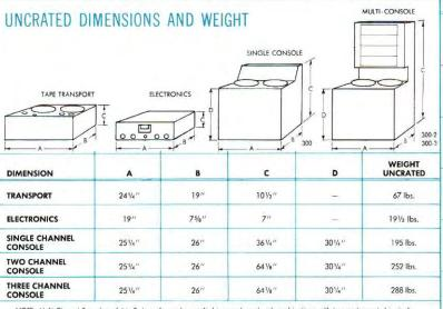
NOTE: Multi-Channel Recorders of 4 to 8 channels may be supplied in console and rack combinations, with transport mounted in single channel console and electronics in separate rack.
